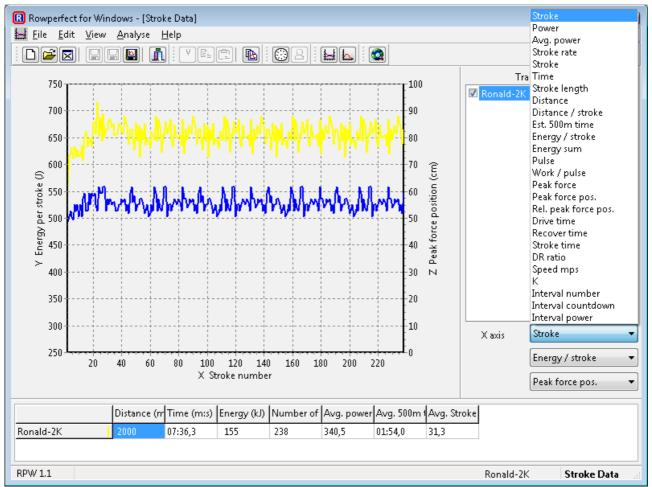
Figure 16 - Stroke data window
