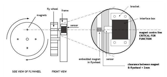
Figure 1 - Interface set-up
