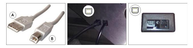
Note : Ensure the orientation of the B connector is correct (and not upside-down).
