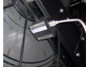
the USB cable provided by plugging in the A connector into a free USB port on the computer, and the B connector into the left side of the ROWPERFECT3 or the RP3 USB Interface.
